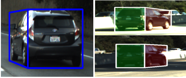
Figure 6. Left: Typical annotation of a car using a rear rectangle and a trapezoid for the side. Note the shared edge reduces the number of required points to six. Right: Visible difference in orientation of the upper side edge.
